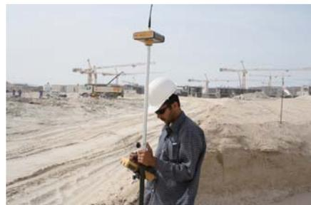
greatly enhanced survey speed and accuracy. Even with the time allotted to establish our own RTK CORS network at this site, we were able to accomplish this challenging task without any delay. It proved how Topcon's RTK-GPS increased productivity." Ibrahim explains.
