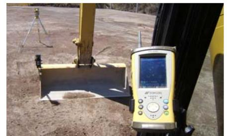
was to set the stakes and strings onto the rock grounds or steep slopes. With this innovative system, we can work without any string, enabling us to complete the excavation with fewer workers in far less time."
