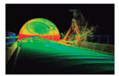
become much more efficient. Also, for other works, the highly-density 3D scanned data is used for designing the alignment, cross section and the ground plan. We believe IP-S3 HD1 can be used not only for road maintenance but also disaster inspection, ageing facility inspection, remodeling progress inspection, before/after the construction comparison, etc."
