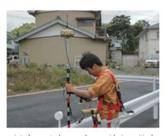
points for control survey by considering critical factors such as sky visibility, radio signal conditions, and accessibility.
