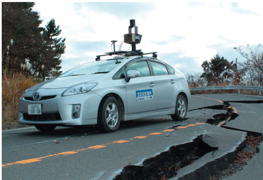
Sato Giken conducted road crack assessment in shorter period of time, which contributed much to the quick disaster recovery.
